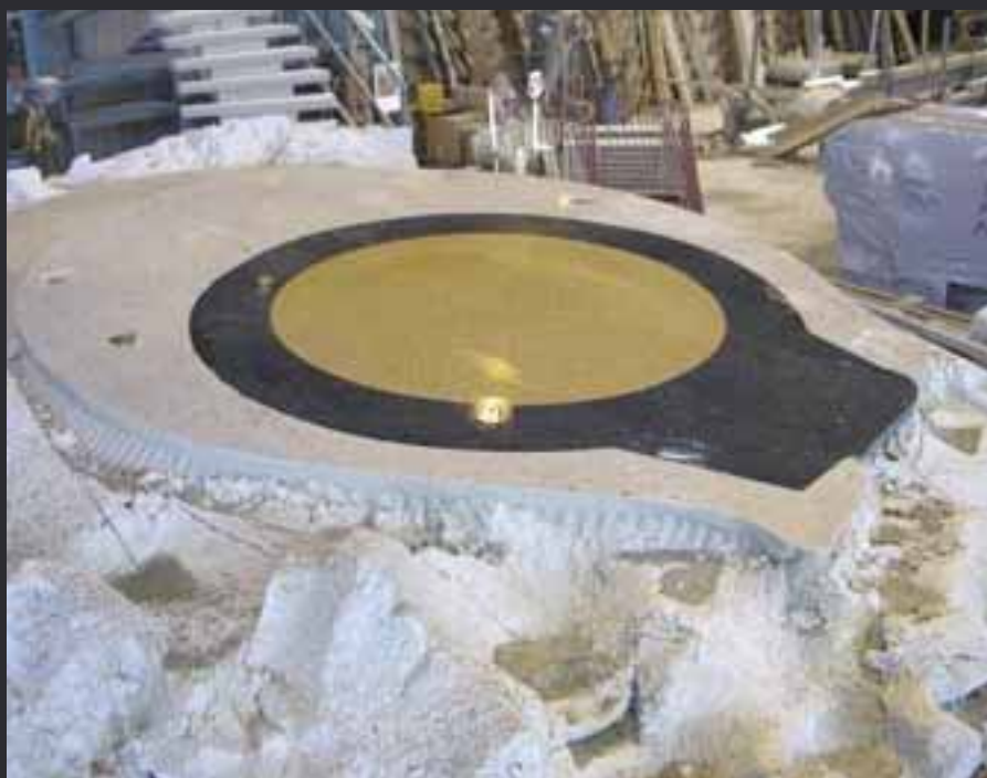
The mould was milled in glued together styrofoam blocks. A void was generated inside the basic shape, which was cast in white concrete, to give lower weight and removal of hydration heat.
