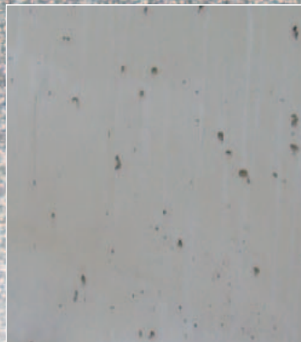
The surface of road barriers normally exhibits blowholes to some extent, as seen on the left. Using the developed SCC, the customer now obtains a perfect surface finish each time, as seen on the right.
