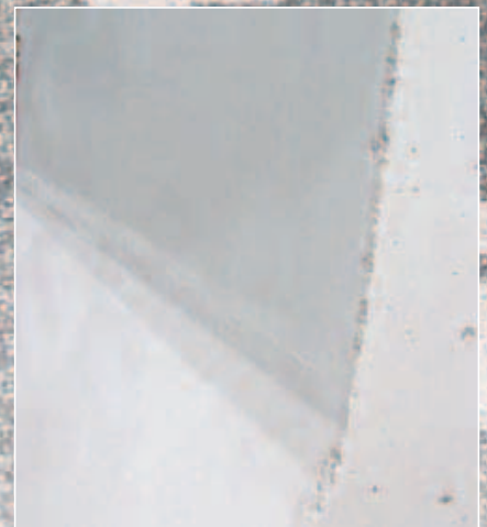
The surface of road barriers normally exhibits blowholes to some extent, as seen on the left. Using the developed SCC, the customer now obtains a perfect surface finish each time, as seen on the right.
