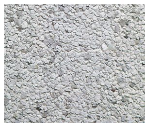
White concrete with exposed calcined flint.
