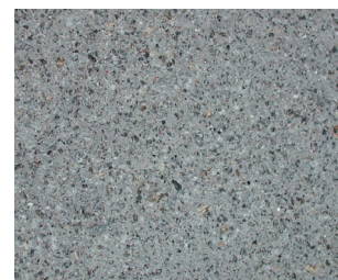
Acid-etched surface with Bayergrün 10/20 (German aggregate).
