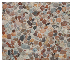
Exposed surface with fine pebble gravel 16/32.
