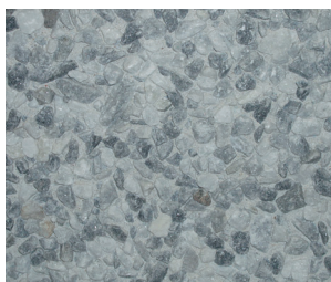
Exposed surface with Hardeberga granite.
