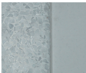
Polished and acid-etched surface with lysite.
